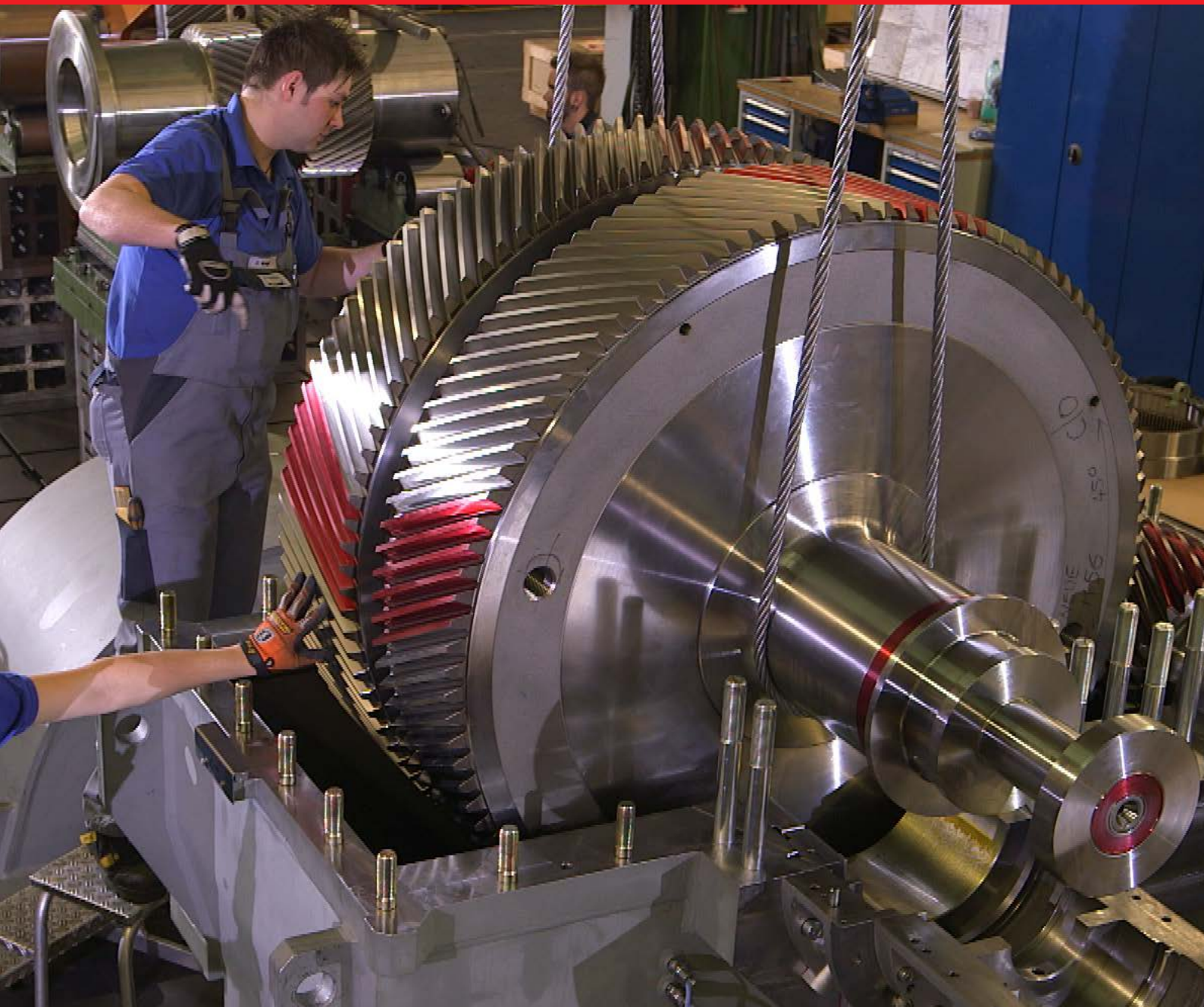
TA71 Gear unit being assembled
